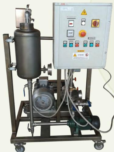
The innovative technology is composed by a cylindrical cavitation chamber: during high speed rotation, rotor channels are periodically aligned with stator channels. The processed liquid is accelerated in the radial direction and flowing through the free channels is subjected to a pressure wave resulting in cavitation.
