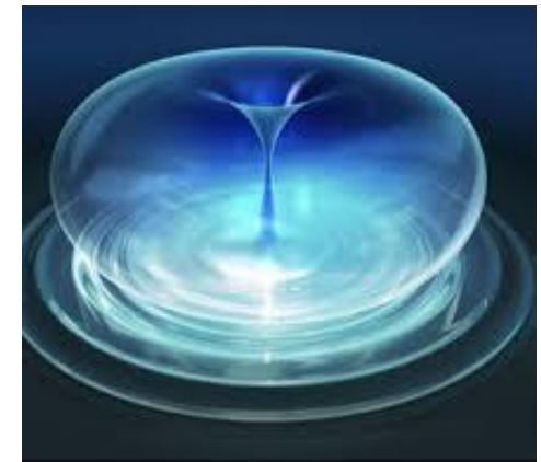
Fig. 1 - Illustration of an imploding cavity in a liquid irradiated with ultrasound
